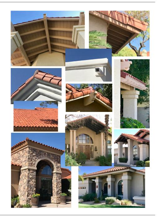
Exterior Walls and Columns: All homes have stucco walls. The finish texture is generally lace in a medium to heavy pattern or smooth. In some cases, full height and/or wainscot stone veneer has been applied around garage doors and on entryway walls and columns.
