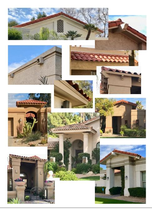
Exterior Walls and Columns: All homes have stucco walls. The finish texture is lace in a medium to heavy pattern. Few homes have wainscot and/or full-height, stone veneer over columns/pilasters, within bays and around garage door openings.
